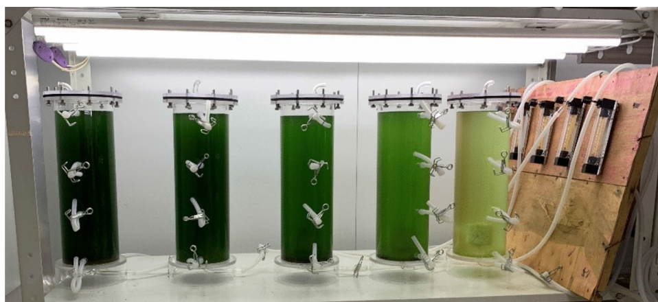
Fig. 1 An algal–bacterial consortium, at a concentration of 500 mg L -1 , showing the bioreactors made on transparent organic glass with a volume of 6 L. The air inlet is located at the bottom of the bottles, and the air outlet is at the bottom. The culture was mixed with a natural algae community and activated sludge in different ratios, as reported by Qi et al. (2021). The selected proportions of sludge and algae were 1:10, 1:5, 1:1, 5:1, and 10:1. All the samples were cultured in the same aerobic wastewater in the photobioreactors for 48 h.
